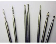
Ensure you have; Drills 0.9mm 1.1mm. Ball bur 0.7mm & 1.5mm. Bud bur 2.5mm. Hart bur 1.8mm. Tapered bur 1mm
