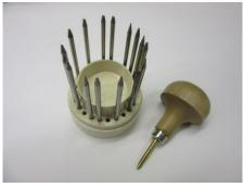
You will need a beading set to perform final claw tip shaping. A video is included showing how to prepare gravers and make other setting tools
