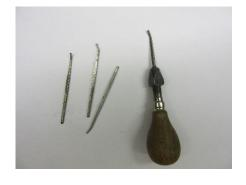
The edge of the setting is finished off with a mill grain effect. This is a matter of choice. The size used is #13. The tool can be held in a pin vise
