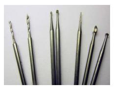
Ensure you have; Drills 0.9mm & 1.2mm. Round burs 1.2mm 1.5mm & 1.7mm. Tapered (fissure) bur 1mm. Hart bur 1.3mm & 1.8mm or tapered setting bur 1.5mm & 2mm
