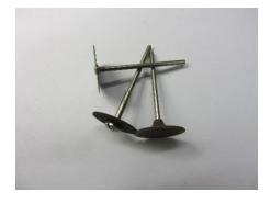
I recommend that you have a brownie and greenie clean up disk for polishing the cut work. For cutting and shaping steel for tool making you will need a separating disk & shaft or a diamond disk
