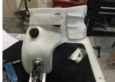
**Design 2: Rolled silicone insert.** Revofit<sup>™</sup> for macro- and micro-adjustability. This design used Click's Lacer HP Releasing Kit (SKU# OK0150-300-05) laminated to the frame for easy on/off. No dummies exist for HP guides, which you must clay up and laminate directly to frame.
