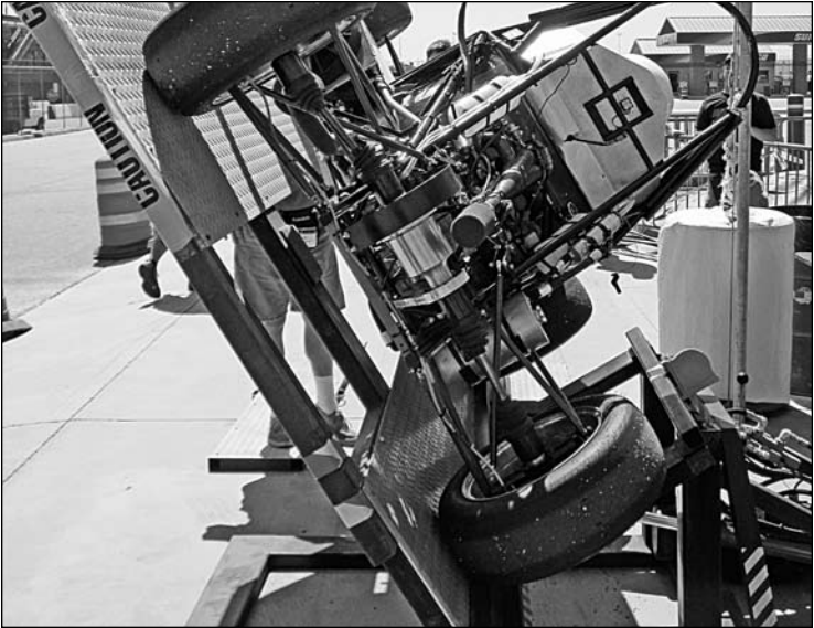
MIT’s FSAE car undergoes lateral load stability testing. It sits unsupported on a 60 degree incline, simulating a 1.7g corner.
