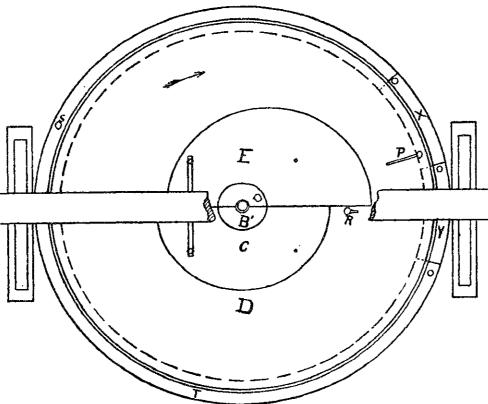
would not only obstruct the freedom of the water flow, but also would tend to lower the richness of the middlings and concentrations by being carried beyond the apartment for the tailings. The trouble was remedied by Prof. Richards screwing on to the edge a strip of wood with its upper edge rounding. This worked much more satisfactorily. There is no doubt but that we could have fed on much more ore if this had been put on at the start.
