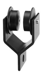
The M-140 Carrier is self guiding with the flanged wheel design. The rollers are made of Delrin, an engineered plastic with excellent properties for use as bearings. The steel axle is machined to a 30 micron finish for smooth rolling under load. The 1.5" long body is made of 1/8" thick 6061T-6 aluminum alloy. Safe working load 25 pounds. 3/8" diam hole for attaching s-hook or trim chain. Available in black or aluminum finish.
