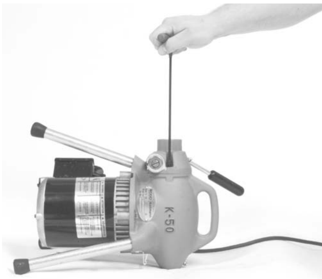
Figure 10 – Retrait des vis Allen
