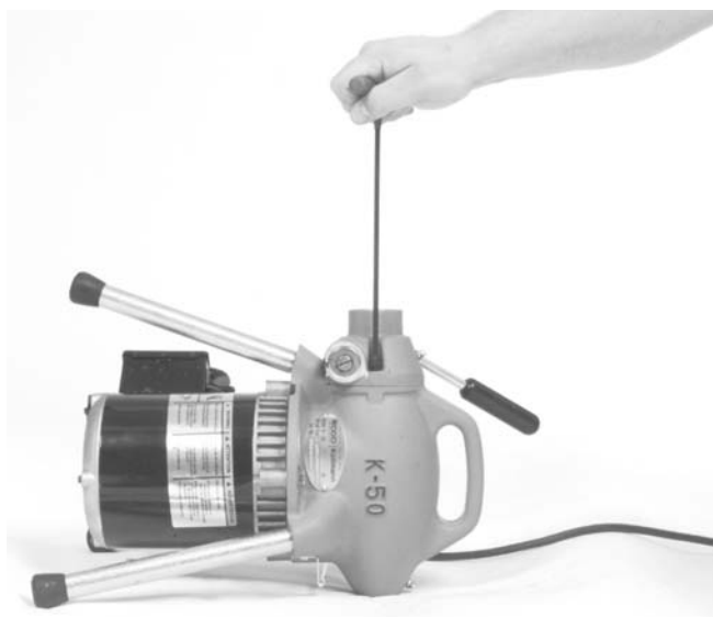
Figure 10 – Remove Socket Head Cap Screws
