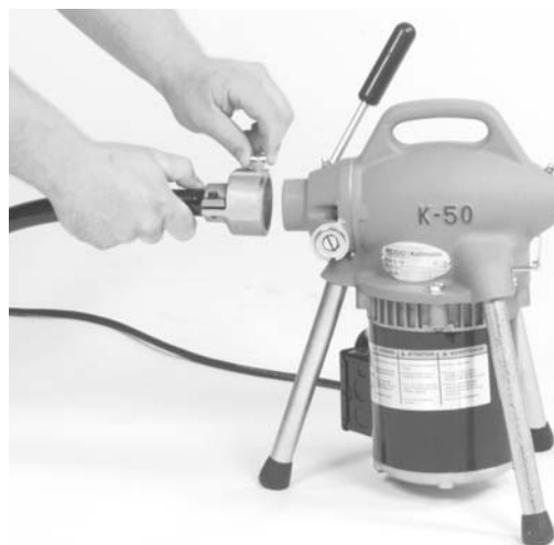
Figure 2 – Rear Guide Hose Attachment
