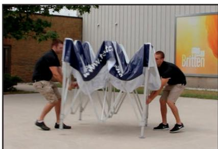
Each person will grab the center scissor piece on their side of the tent frame and pull it away from the center by walking/pulling backwards. Move the legs outwards until the scissor pieces are fully extended.
