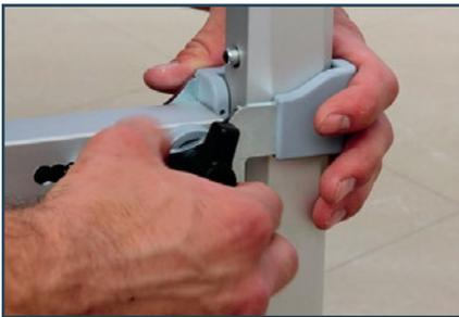
To attach the half-wall bar to the tent legs, twist off the black knob on the outside of both clamps and remove the L Clamps. Place the L clamp attached to the half-wall bar on both tent legs directly below the push buttons on the legs.
