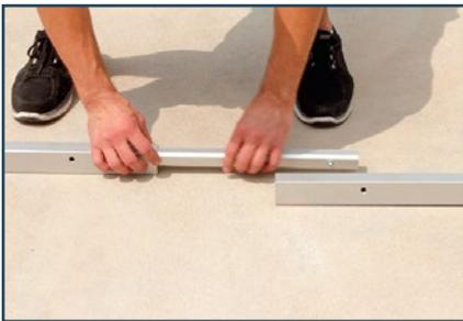
Press the push button on the connector piece in and slide it into the longer half wall bar until it snaps into place. Repeat this step with the push button on the opposite end of the connector bar. The result is one long half-wall bar with clamps at both ends.
