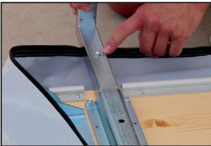
Prepare the counters for installation by removing the first metal leg from bracket on the underside of the counter. Flip the leg up so the shorter end with the push button is parallel to the counter. Press the push button in and slide the leg into the metal bracket until it snaps into place.
