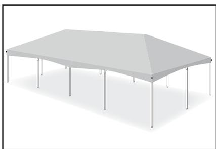
Finish by installing the legs in the final two intermediate brackets on the 20' sides. Make sure all snap pins are locked in place.
