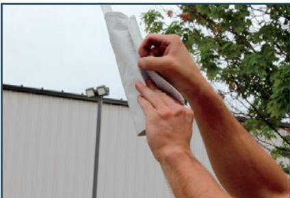
Once the tent is secured to all water barrels, fold the extra out guy strap length into the white vinyl covers with Velcro closure.
