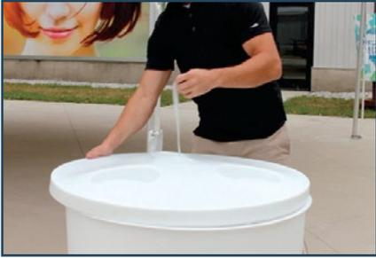
Place the top onto the barrel, making sure to run the outguy strap through the hole in the top.
