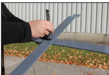
Align the holes in the middle of both cross base arms and insert the flag spindles into the hole from the top. Twist the spindle until it securely holds the two arms together.
