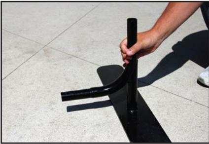
Insert the bottom corner bracket into the top of the footplate. Repeat for both left & right footplates.
