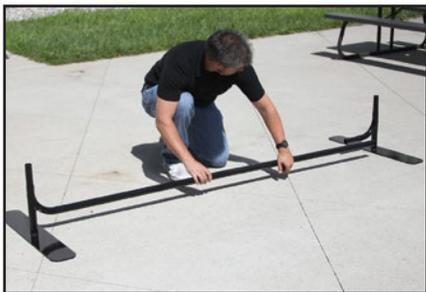
Insert the bottom pole section into both the left and right bottom corner brackets.
