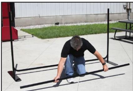
Locate a 4'-A pole and a 4'-B pole and insert them into one another to create the top pole section.
