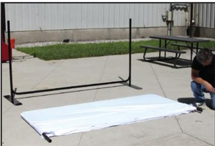
Slip this cover over the top pole section, leaving 6" of the left & right 4' poles exposed.
