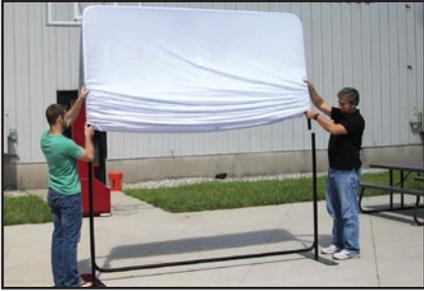
Grab top pole section from both left & right sides. Lift section up and place down into the base section.
