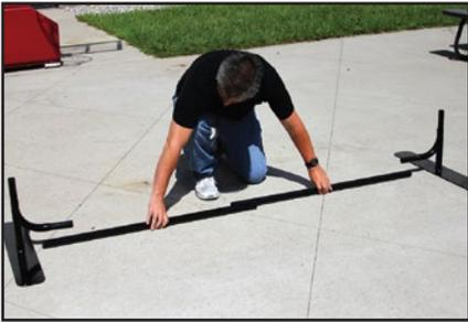
Lay a 4'-A pole and a 4'-B pole end to end between the footplates on the ground.
