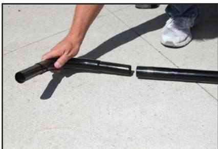
Insert the top corner bracket onto the end of the top pole section. Repeat for both the left & right sides.
