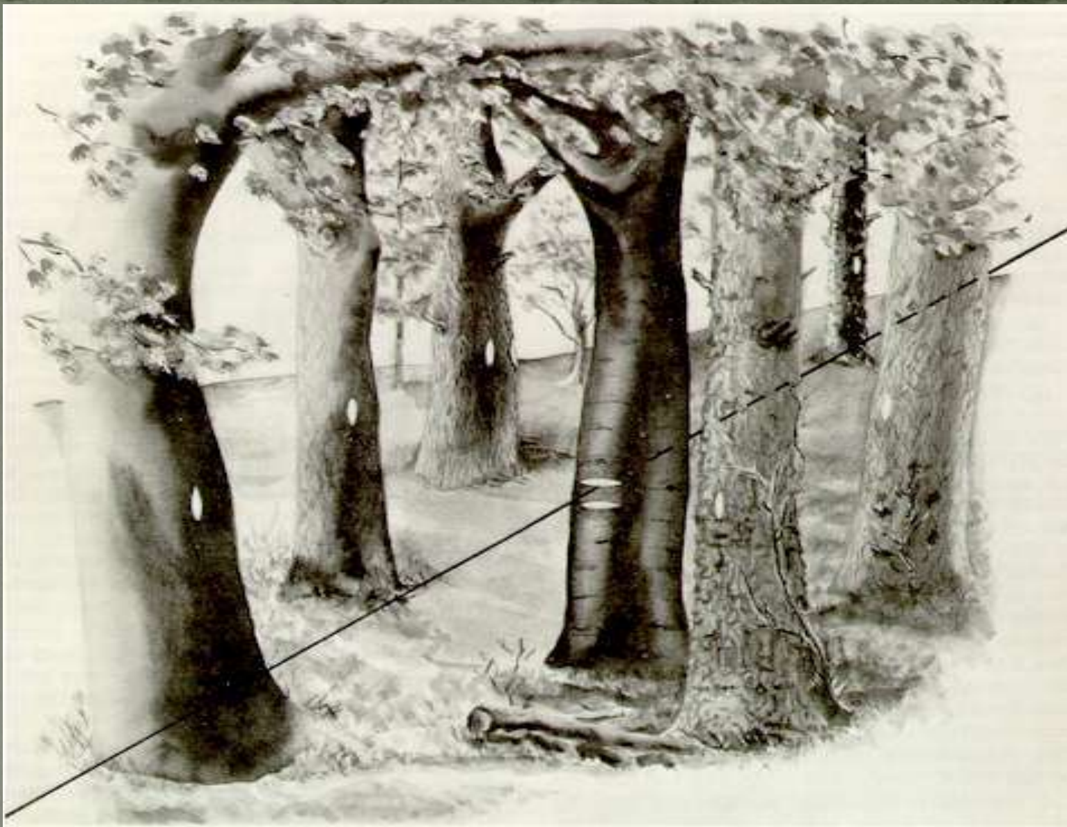
FIGURE 63. - Marking a line through timber.
