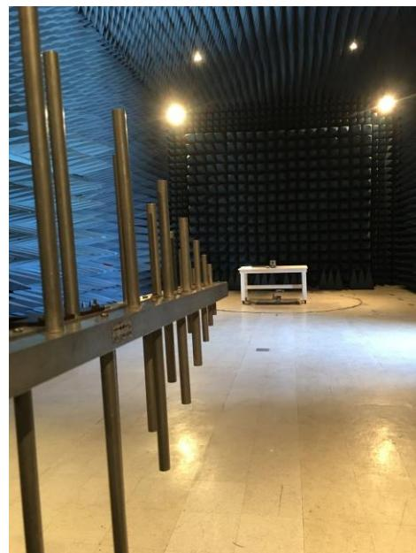
**Radiated Emission Set-up for 0.02 – 1 GHz**
