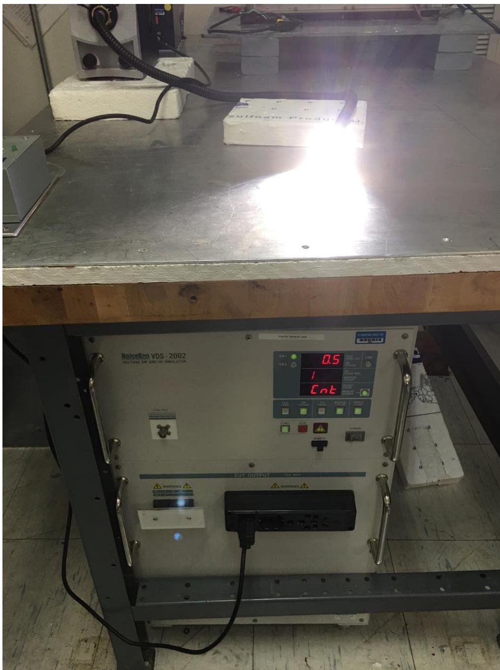
**POWER LINE DIPS AND BROWNOUT TEST SETUP**
