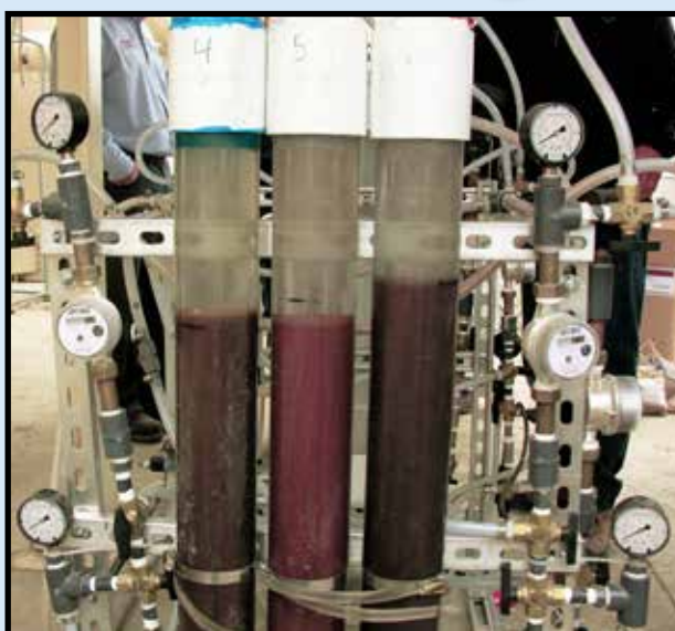
Pilot Stand Vessels 4 - 6 @ 0.25 gpm
