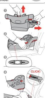
A This child restraint base is designed to be used with lower LATCH anchors at the standard spacing (11 inches) ONLY! Refer to vehicle owner's manual for information about LATCH and child restraint installation positions.
