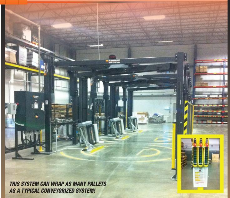
Wraps 3 pallets at one time. 80-90 pallets per hour!
