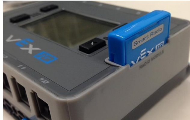
Smart Radio INCORRECTLY Installed
