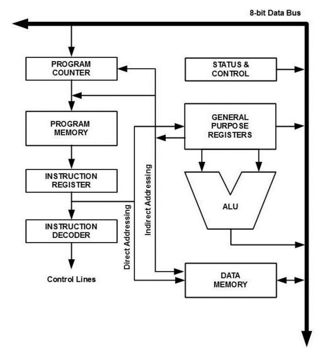
Figure 4 - Architecture of AVR core
