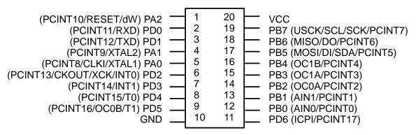
Figure 1 - ATtiny2313A pinout
