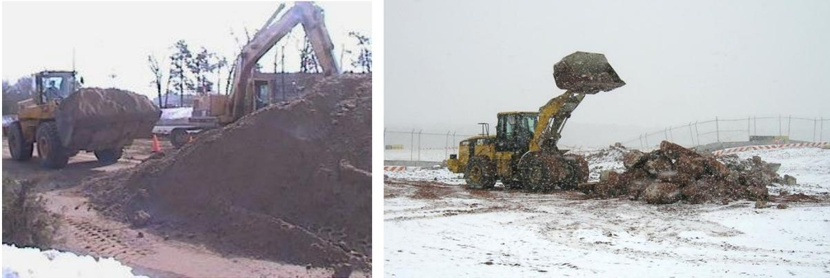
Loaders are one of the most versatile pieces of equipment at any Heavy Civil Construction Project and therefore they are found on almost every site. Some are tractor-loader-backhoes, although most are straightforward front-end loaders.
