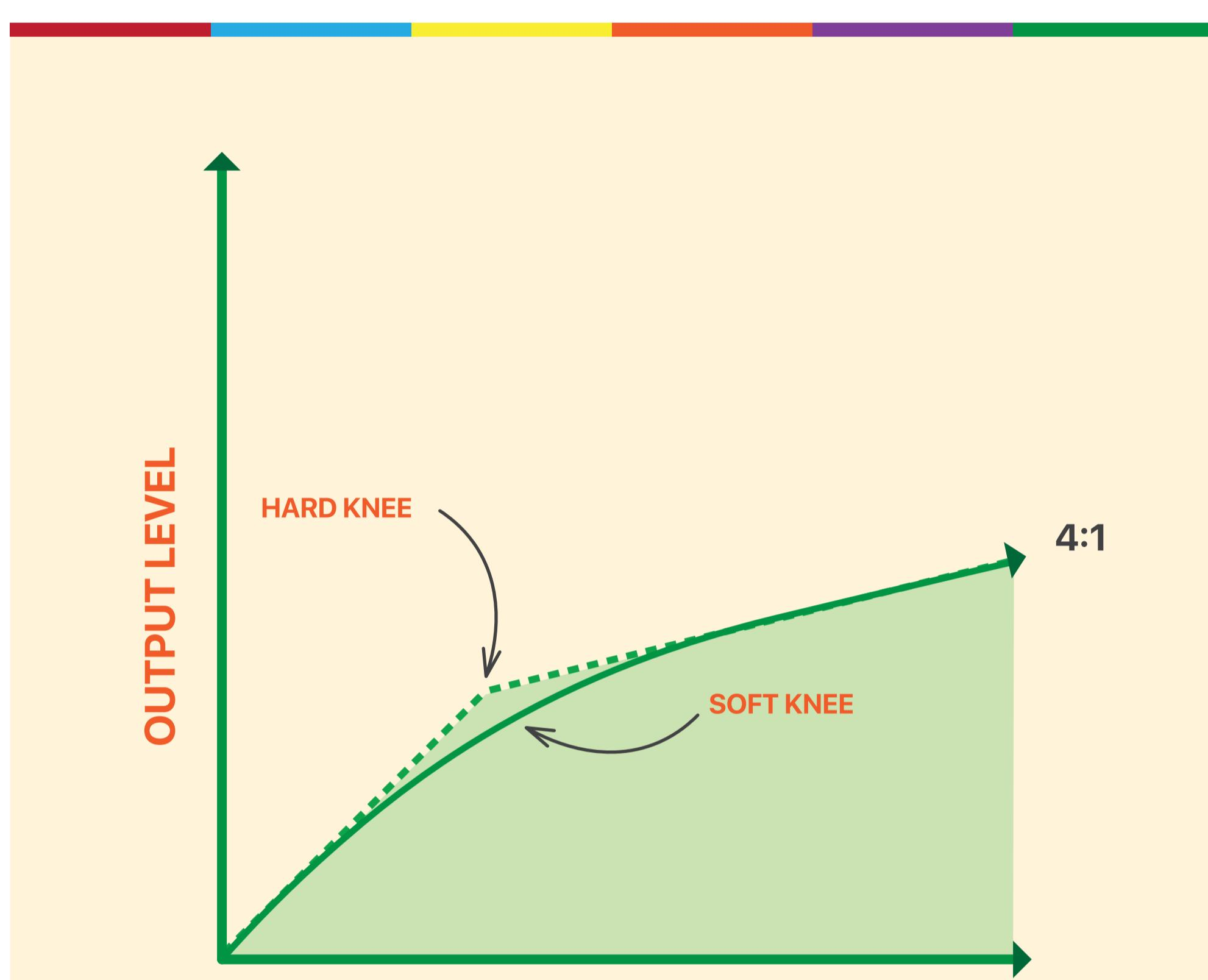
Most compressors have a knee setting, and it's also another control that helps dictate how hard the compression is.
