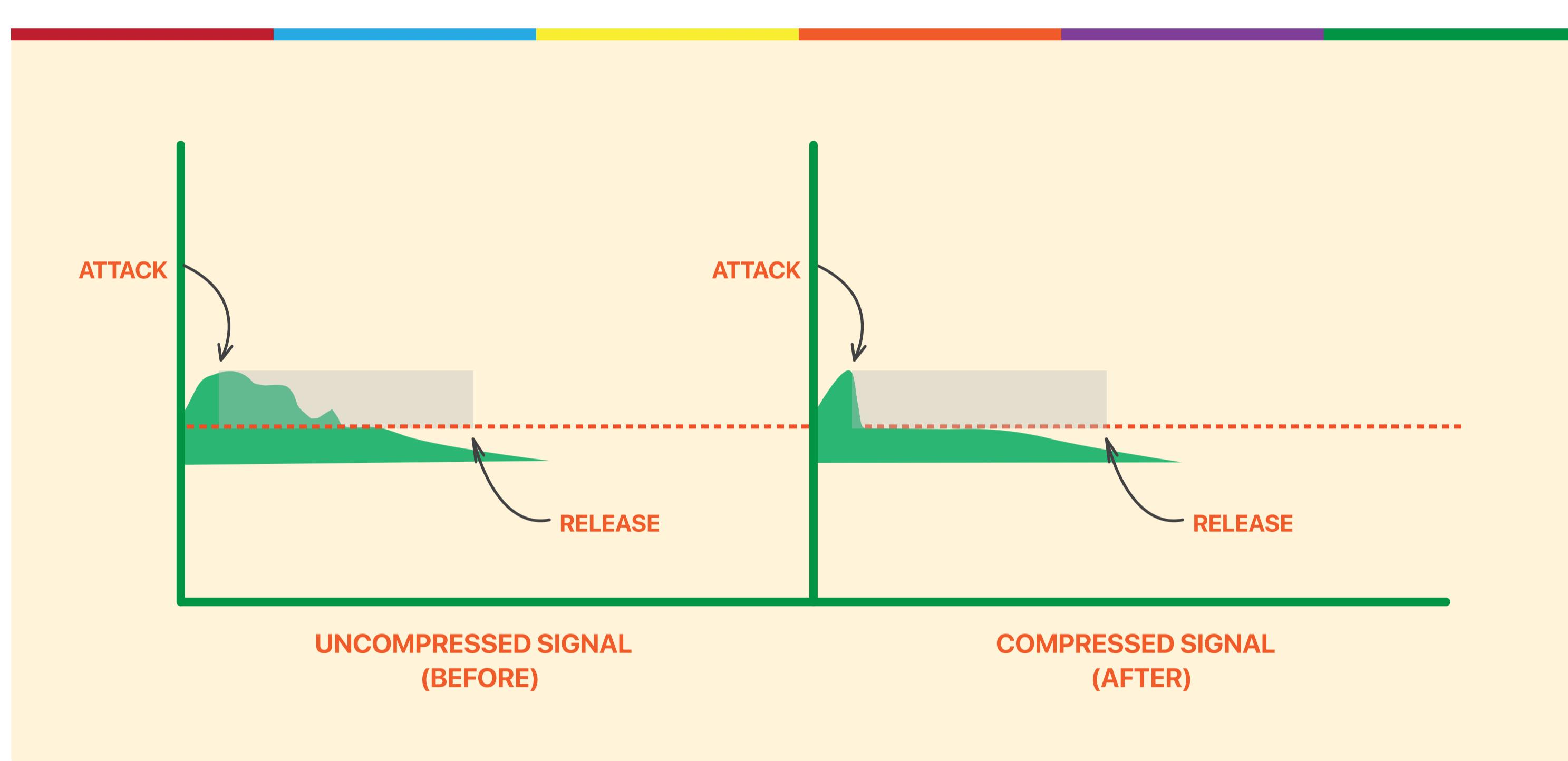
A slower attack will allow fast material to come through clearly, such as the aforementioned transients, before the compressor engages and brings everything down.
