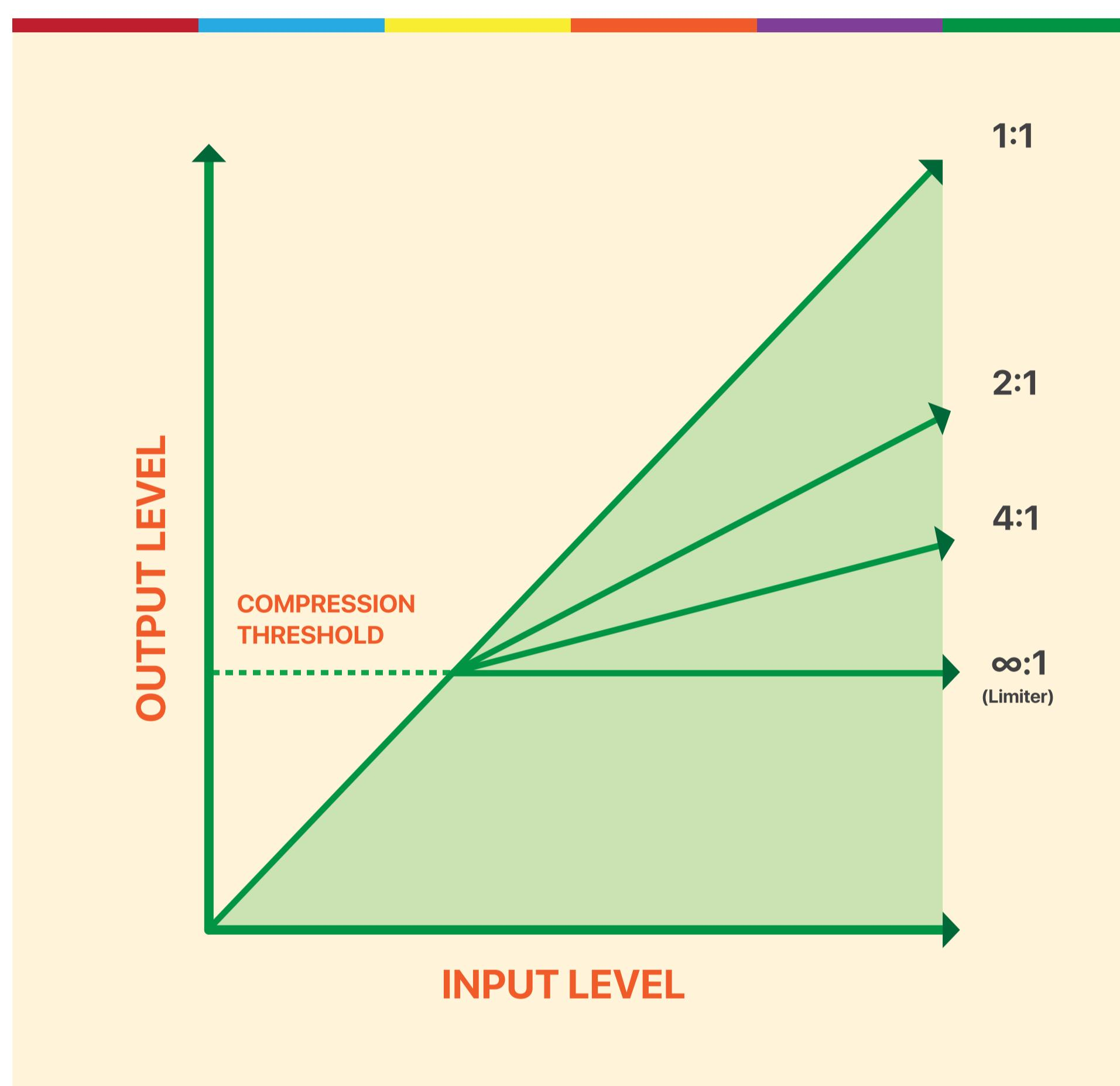
**Note:** A ratio of 1:1 would have absolutely no effect on the input signal.
