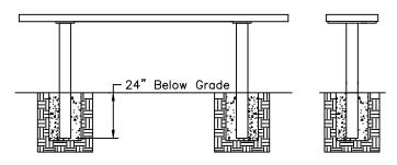
ALL SEAT BRACKETS AND FOOT MOUNTING BRACKETS ARE 3/8" X 4" BAR STOCK
