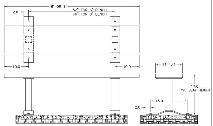
FRAMES SHOULD BE ANCHORED TO A CONCRETE PAD PROVIDED BY THE CUSTOMER
