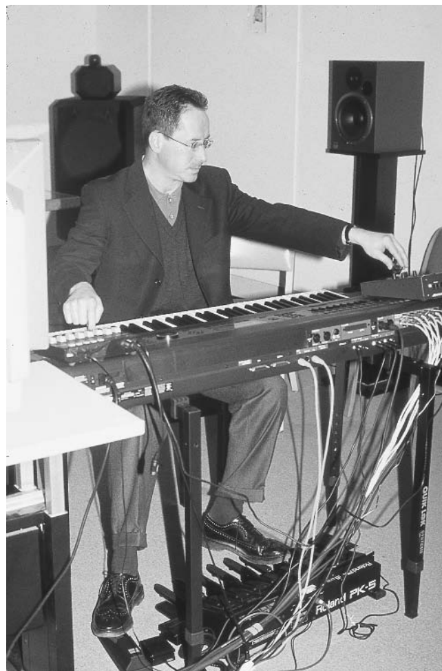
Figure 5.3 The author playing the Creatovox synthesizer in CREATE's Studio Varèse, January 2000. The physical hardware consists of a MIDI keyboard controller, MIDI joystick, and footpeds. A Power Macintosh computer receives the MIDI data. The Creatovox software interprets the MIDI data and synthesizes the sound, with octo- phonic output through a Digidesign Pro Tools 24 converter.
