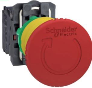
Harmony XB5, Emergency stop switching off, plastic, red mushroom Ø40, Ø22, trigger latching turn to release, 1 NO + 1 NC
