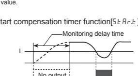
Set monitoring delay time so that there is no output during the delay time.
