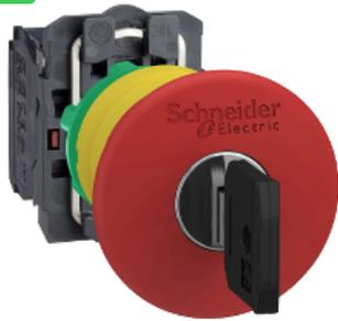
Harmony XB5, Emergency stop switching off, plastic, red mushroom Ø40, Ø22 trigger latching key release, 1 NO + 1 NC
