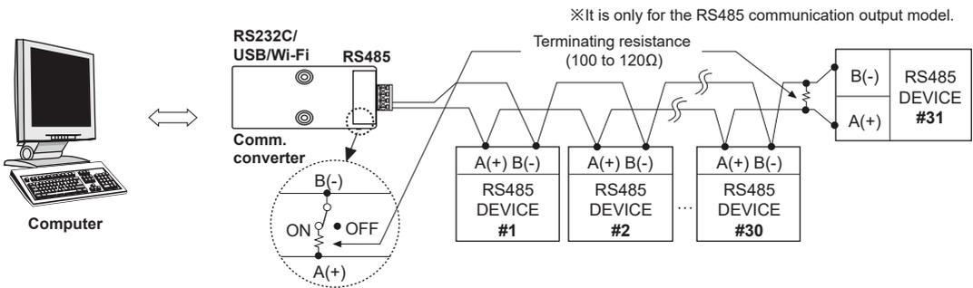
※It is recommended to use Autonics communication converter; SCM-WF48 (Wi-Fi to RS485-USB wireless communication converter, sold separately), SCM-US48I (USB to RS485 converter, sold separately), SCM-38I (RS232C to RS485 converter, sold separately).
