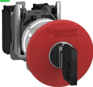
Harmony XB4, Emergency stop switching off, metal, red mushroom, Ø40, Ø22, trigger latching key release, 1 NO + 1 NC
