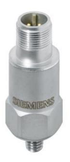
SIPLUS CMS2000 VIB-SENSOR S01 ACCELEROMETER; FREQUENCY RANGE 0,5HZ TO 15KHZ; MEASUREMENT RANGE 50G; SENSITIVITY 100MV/G (+/-10%); MIL-PLUG ON TOP
