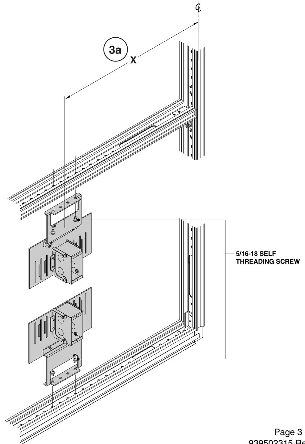
**4.** Remove the desired knockout(s) in the box and add your conduit connector and flex (or rigid) conduit (extra flex conduit is recommended). Run wire and make all electrical connections to the building source. Use cable ties as needed to ensure a prolonged stable support of conduit.
