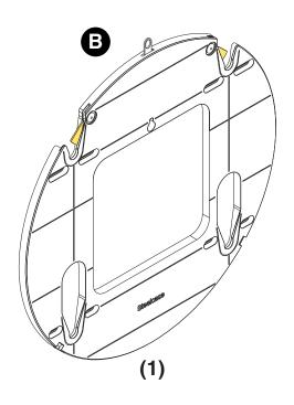
**4.** Tap nail in at top of center keyhole, and aligned with the horizontal markings. Hang the wall mount bracket on the nail.
