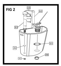
To mount ceramic tank (A7), locate the centerline on the wall behind the bowl and mark tank height using instructions on page 1. We recommend that the bottom edge of the tank (A7) be about 62.5 inches from the floor for a regular 16 inch toilet bowl. Secure tank (A7) and tank spacer (D) to studs using lag bolts (D1). If studs are not accessible, we recommend installing a sufficient backing behind the finished wall to provide a secure material to mount the tank (A7) and spacer (D).(FIG 3)
