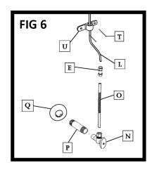
Install the nipple (P) to the water fitting from the wall.
