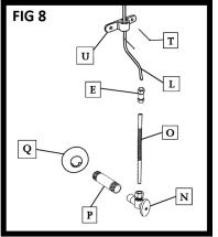
Turn off the shut off valve (N) and fill the tank to its waterline and test the flush system, checking for leaks. Water level is pre-adjusted from the factory and in some cases may need to be re-adjusted. CAUTION: Before turning on water please make sure all parts are secure and installed properly. Never use abrasives, detergent, or acids to clean the unit as they will damage the unit and void the warrenty.
