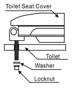
Insert bolts into mount holes on toilet. Secure using washer and locknut.
