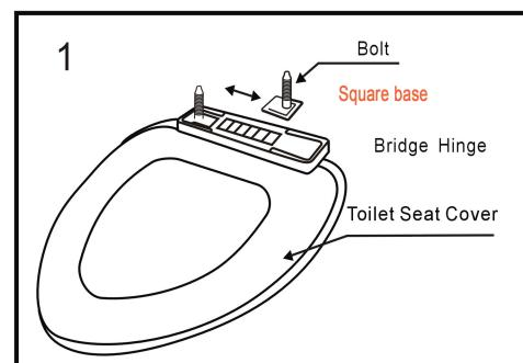
Remove the locknut and washer from the bolt.
