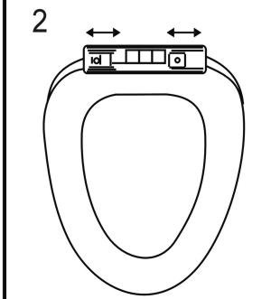
Move the **bolts to** the left and right, adjust the distance between two Bolts to make them match with the Toilet Holes.
