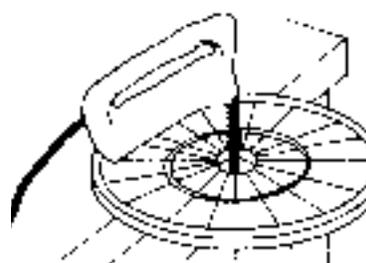
4. For installation around the ceiling pan, cut hole with saber saw, hand saw or serrated knife.
