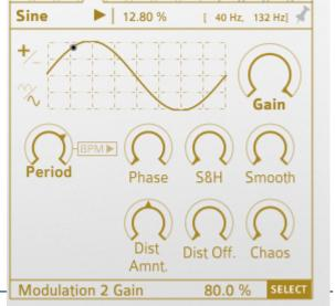
**Distortion Amount** controls the symmetry of your modulation pattern. At default value (50%) your curve is split between equal positive and negative phases. At 25% the first is now three times shorter than the later (25 to 75 ratio).
