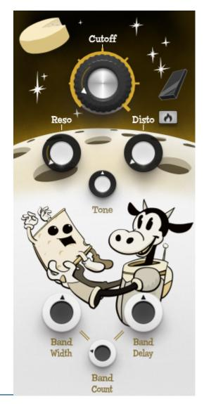
**Band Delay** affects the delay times of all the bands. When it is in the middle position, there is no delay. When the knob is turned to the left, the lower bands are more delayed, and when the Knob is turned to the right, the higher bands are more delayed.
