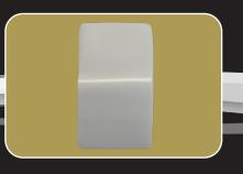
Stress whitening is really a craze, which is a pre-cursor to a crack. As the material is stressed, micro-voids are formed and polymer chains (fibrils) link the two sides of the craze. Because the refractive index of the craze is different than the refractive index of the base polymer you 'see' this as the whitening effect (see image below).
