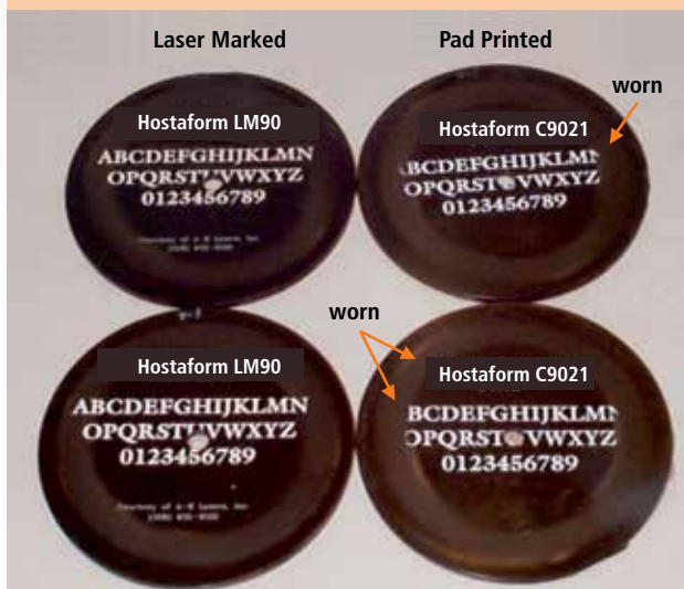
Fig. 92 100 cycles of Taber abrasion, CS-10 wheel, 1000g weight
