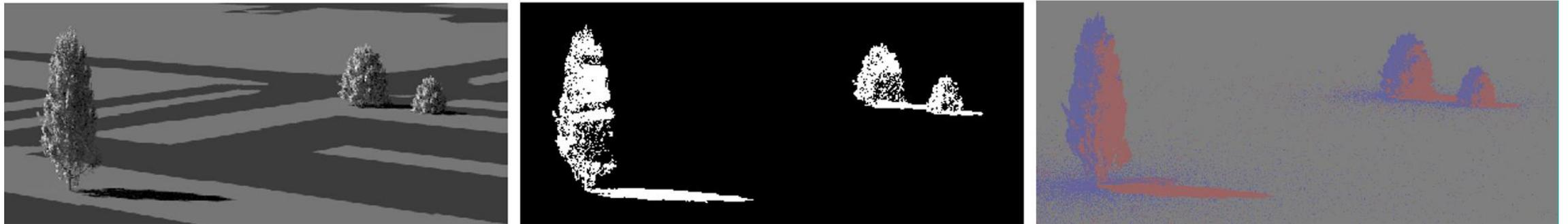
Simulated DIRSIG scene with trees (left) and an occlusion and shadow mask ground truth image (center) showing all occluded and shadowed pixels in the scene in white. On the right is the result of a spectral angle classification that is used to detect change between the initial ground terrain image and a simulated observed image frame containing trees
