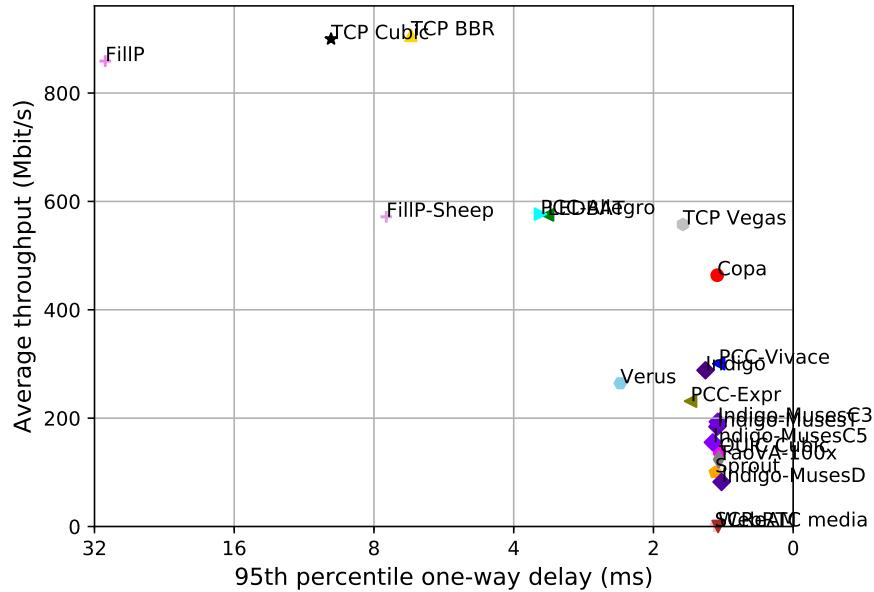
test from Stanford to AWS California 1, 5 runs of 30s each per scheme
