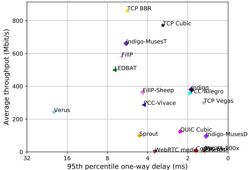
test from AWS California 1 to Stanford, 5 runs of 30s each per scheme
