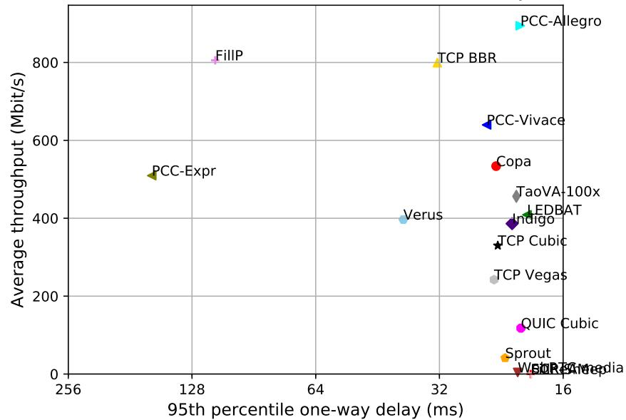
test from AWS California 1 to Stanford, 10 runs of 30s each per scheme
