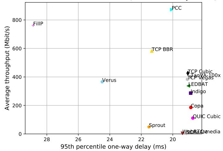
test from AWS California 1 Ethernet to Stanford Ethernet, 10 runs of 30s each per scheme
