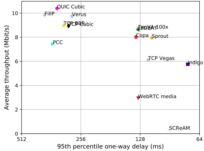
test from Stanford ppp0 to AWS California 1 Ethernet, 3 runs of 30s each per scheme
