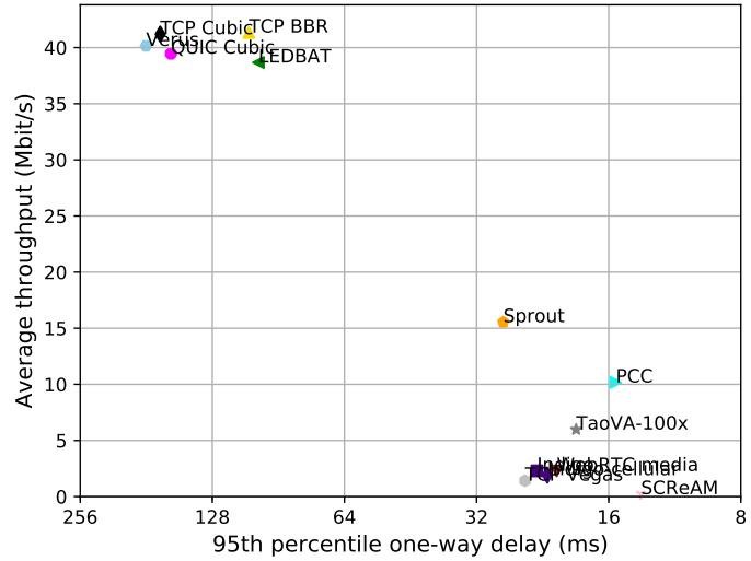
test from AWS California 1 Ethernet to Stanford ppp0, 3 runs of 30s each per scheme
