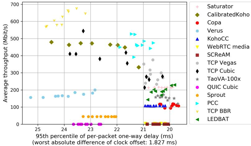
test from AWS California 1 Ethernet to Stanford Ethernet, 10 runs of 30s each per scheme
