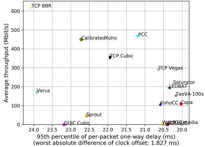
test from AWS California 1 Ethernet to Stanford Ethernet, 10 runs of 30s each per scheme
