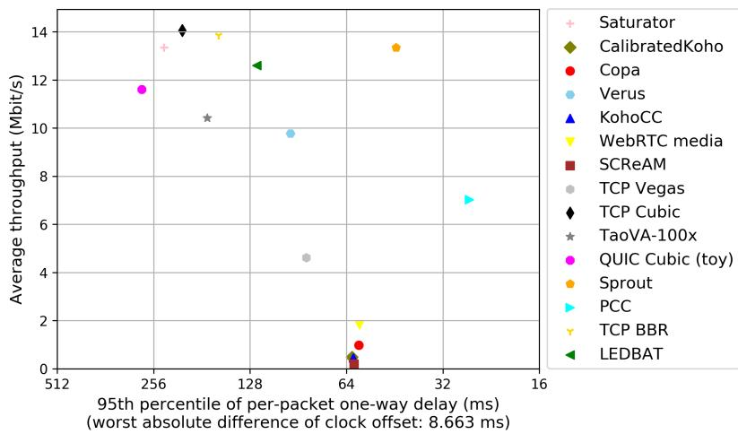
test from Stanford ppp0 to AWS California 1 Ethernet, run 1 of 30s each per scheme
