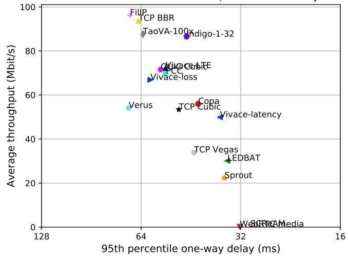
test from AWS California 2 Ethernet to Mexico Ethernet, 10 runs of 30s each per scheme
